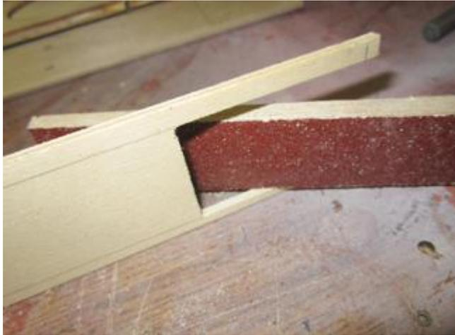
For neat and straight edges on parts I cut for my airplanes, make custom-sized sanding sticks to fit into tight areas. Simply get some stick-on sandpaper (usually for electric sanders) and cut it into strips. Make your sanding stick to fit and then apply the sandpaper. The result is clean edges for a professional-looking job.
