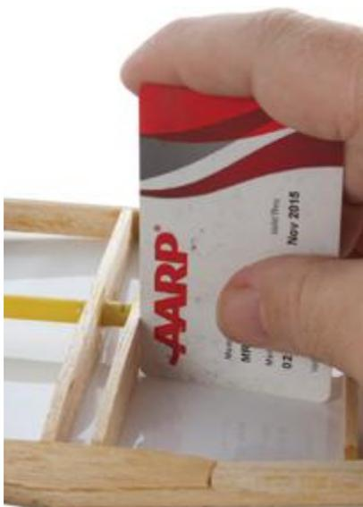
Here is the way to use your old credit cards and build straight at the same time. While building wing panels on plans, you have to ensure the ribs are 90 degrees to the building board. Old plastic credit cards are great building guides as their edges are perfectly square and the corners are rounded so they don't get glued to the rib during construction. When they get ratty, just throw them away.
