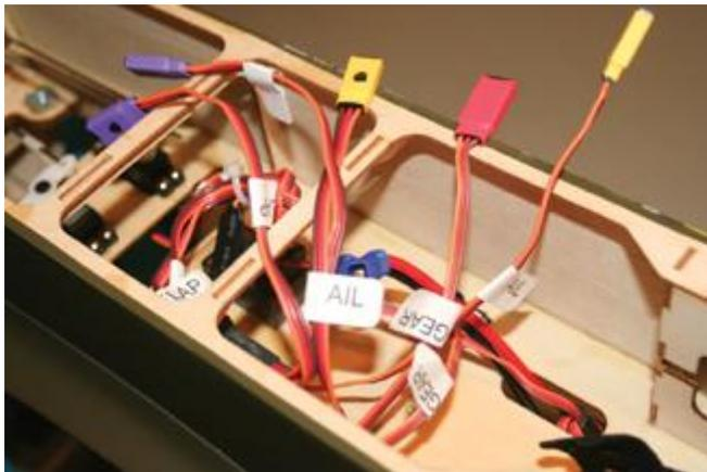
At times even when servo labels stay on, it is much too tedious to plug them all in properly. To solve this, buy several different colors of heat-shrink tubing: 3/8 inch for the female connectors and 1/4 inch for the male. To make it easy to determine the correct polarity, draw dots on the tubing with a felt-tip marker to make connecting them a snap.
